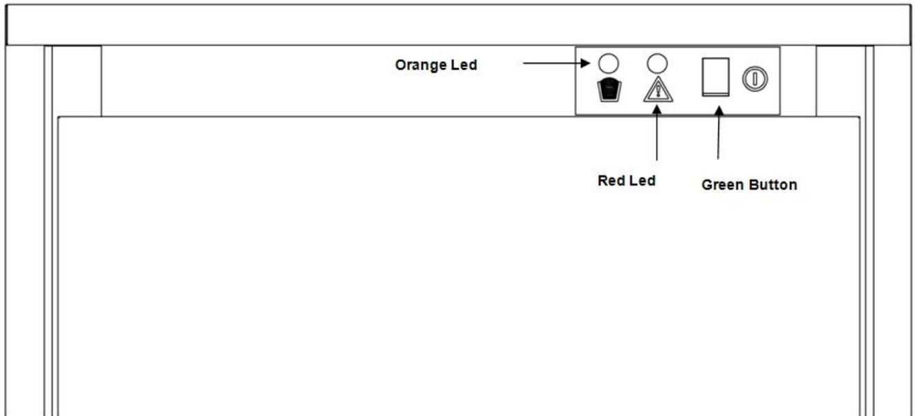
**Green button:** Starts the machine. It is indicated with the led on.
