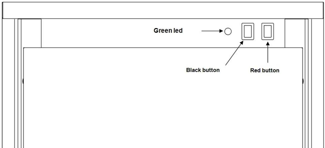
**Green led:** Shows that the machine is activated. The machine might be stopped by the stock thermostat.
