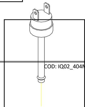
This safety device trips when pressure is too high. Pressure might reach the set limit of 27 Kg/cm<sup>2</sup> when:
