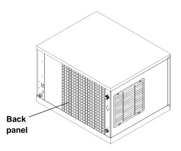
3) Clean condenser using a vacuum cleaner, soft brush or low pressure air. Clean from top to bottom, not side to side. Be careful not to bend the condenser fins.
