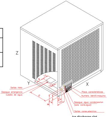
Ice discharge slot. Water trough overflow
