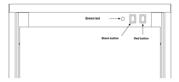
**Green led:** Shows that the machine is activated. The machine might be stopped by the stock thermostat.
