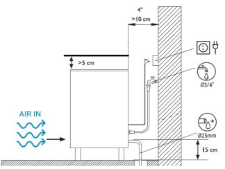
Exits/renewals of the air between the rear of the machine and the wall must be provided for.
