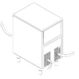
THREAD THE SUPPORT LEGS TO THE BASE OF THE MACHINE ON THE HOUSING SET TO SUCH END AND REGULATE THE HEIGHT AS TO HAVE THE EQUIPMENT PERFECTLY LEVELED.
