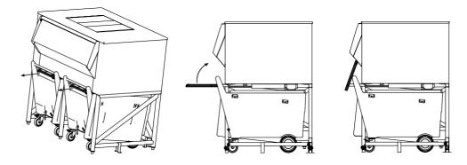
Once the cart is full enough, place the gate back in its original position, cutting off access for the ice. To do this, lower the handle and push the gate back inside as far as it will go.
