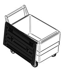
With the lid off, place the cart under the ice storage bin. Check that the cart is pushed all the way to the very end. Its front wheels should touch a tube as shown in the figure.
