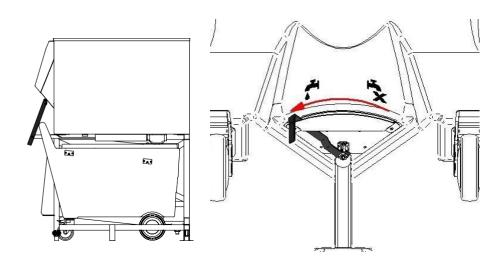
Once all the water has drained out of the cart, close off the valve.
