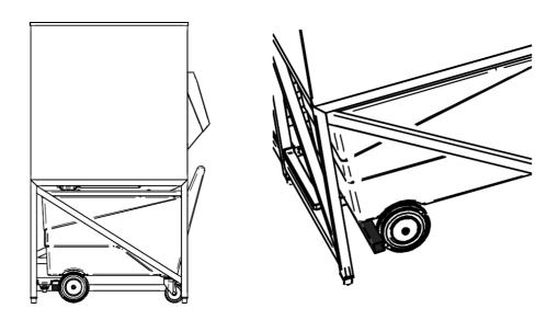
Immediately after, lock the wheels of the cart. To do this, lower the levers on the rear wheels of the cart. Use your foot to press the levers down.
