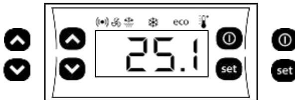
Access and use of the menu to adjust the temperature of the equipment:
