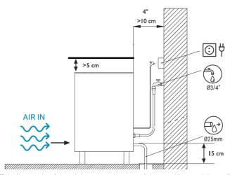
Exits/renewals of the air between the rear of the machine and the wall must be provided for.
