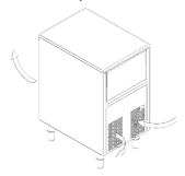
THREAD THE SUPPORT LEGS TO THE BASE OF THE MACHINE ON THE HOUSING SET TO SUCH END AND REGULATE THE HEIGHT AS TO HAVE THE EQUIPMENT PERFECTLY LEVELED.
