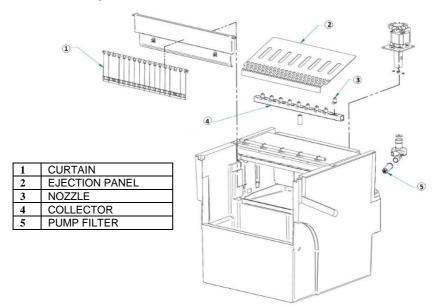
**CAUTION:** IT IS VERY IMPORTANT WHEN REPLACING THE CONTAINER THAT THE NOZZLES ARE PERPENDICULAR, AS IF TWISTED, THE EXTERNAL CUBES COULD RUN OUT OF WATER.
